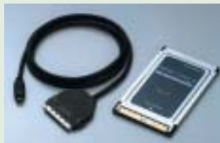
DS-0297 Interface card / cable for PCMCIA (Card Bus)
